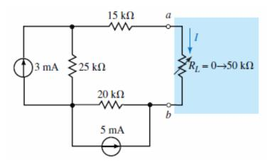
17. a.  $R_{\text{Th}} = 60 \text{ k}\Omega$   $E_{\text{Th}} = 25 \text{ V}$ b.  $R_L = 0$ : I = -0.417 mA $R_L = 10 \text{ k}\Omega$ : I = -0.357 mA $R_L = 50 \text{ k}\Omega$ : I = -0.227 mA
