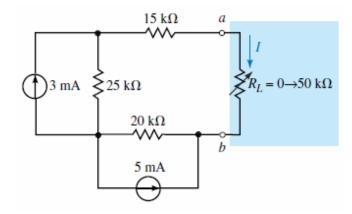
33. a.  $I_N = 0.417 \text{ mA}$ ,  $R_N = 60 \text{ k}\Omega$ b.  $I_N = 0.417 \text{ mA}$ ,  $R_N = 60 \text{ k}\Omega$
