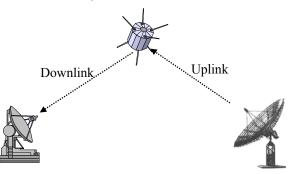
Figure 1-14: Satellite Transmission
