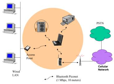
Figure 1-11: A Simple Bluetooth Configuration
