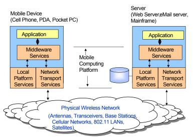
Figure 1-5: Platforms for Mobile Applications
