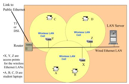
Figure 1-10: A Sample Configuration with Wireless Ethernet LANs
